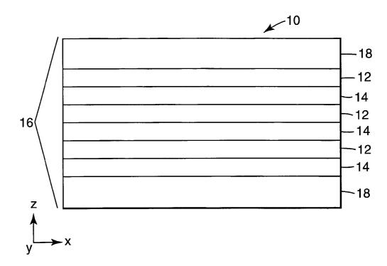
(57) Abstract: Modified copolyesters having relatively low refractive indices and relatively high glass transition temperatures are disclosed. These modified copolyesters can be used in forming one or more layers in an optical film, such as a multilayer polymer
