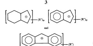
where R" is alkyl from  $C_1$  to  $C_{20}$  and q is 0 to the maximum number of substitutable positions such that there is at least one H remaining on the cyclopentadienyl ring. The reaction 15 forms  $MX_m$  and a polymeric oil having the formula
