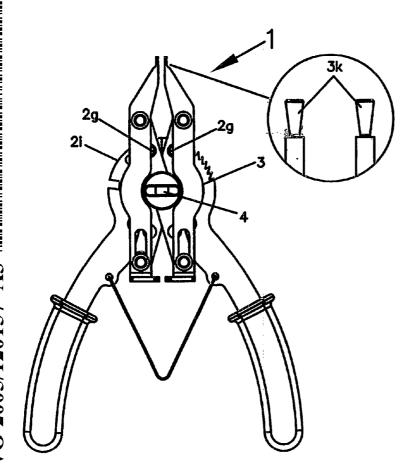
(57) Abstract: The jaw portion (3) comprises cross levers (3a) centrally connected by a rotatable central axis (3f) with a throughbore (3g) and outwardly connected by lever pivots (3e) to parallel jaws (3h) (within clots at one end) with tapered operating tips (3k) at either end.
