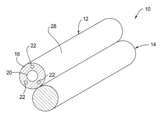
(57) Abstract: The invention provides a fuser apparatus including a fuser roller and a pressing roller. The fuser roller includes one or more heat pipes situated in longitudinal bores in the roller body. The heat pipes are coated with a thermal interface material for conducting heat between the roller body and the heat pipe.
