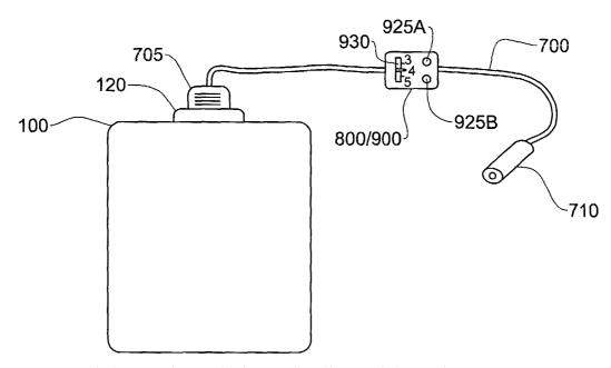
(57) Abstract: A portable charger employs metal air battery cells and has enough charge and current capacity to permit simultaneous use and charging of an attached appliance with a scondary battery. This allows, for example, a cell phone user to use a cell phone for extended periods of time. Preferably, the primary charger may have an extension cord to allow the primary batteries to be located remotely from the appliance, for example attached to a belt.
