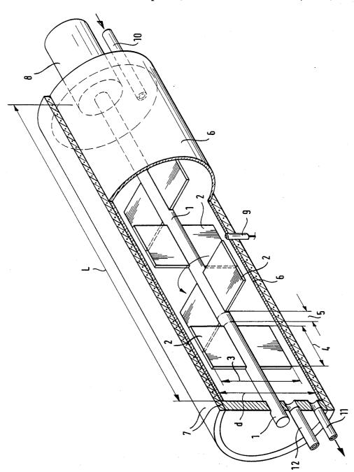
The shaft (1) is equipped with rectangular stirring blades (2) which are staggered at 90° from each other.
