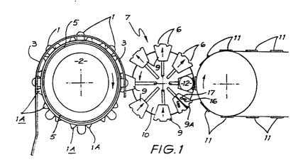
THIS INVENTION relates to poultry processing plant and more particularly to apparatus for transferring slaughtered birds from a first overhead chain conveyor to another such.
