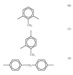
in which the moiety  $R_1$  is of formula (Q) in about 16% of the repeating units, of formula (T) in about 64% of the repeating units, and of formula (S) in about 20% of the repeating units
