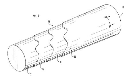
(57) Abstract: A calender roll for a papermaking machine includes: a substantially cylindrical core; and a cover circumferentially surrounding the core. The cover comprises: a base layer circumferentially overlying the core; and a topstock layer comprising polyurethane circumferentially overlying the base layer, the topstock layer being fiber-reinforced, the polyurethane having a glass transition temperature of between about 120 and 150°C, the topstock layer having a hardness of 70 to 90 ShD.
