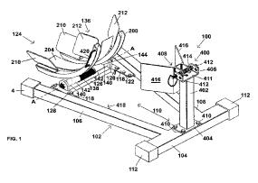
(57) Abstract: An apparatus for supporting a motorcycle in an upright position. The apparatus includes a base and a wheel stop coupled thereto. A cradle is pivotably coupled to the base and includes a pair of clamp members slidably coupled thereto. The pair of clamp members are biased away from each other. In other embodiments, a chock apparatus and a method of holding a motorcycle in an upright, stable position using a chock apparatus are provided.
