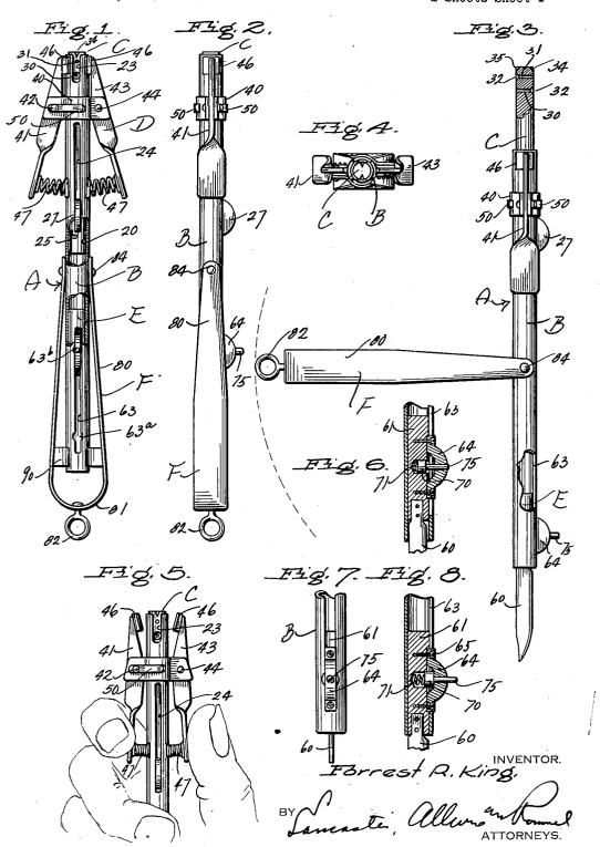
STRAND SPLICING DEVICE AND METHOD Filed Nov. 28, 1947 2 Sheets-Sheet 2 Fig.12.
