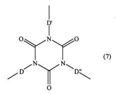
wherein D, D' and D" are, independently, a linear or branched divalent  $C_1-C_{12}$  alkyl radical, a divalent  $C_5-C_{14}$  alkylcycloalkyl radical. Examples triisocyanates include, but are not limited to, the isocyanurate trimer of hexamethylene diisocyanate, 2,4,6-toluene triisocyanate, p, p', p"-triphenylmethane triisocyanate, and the trifunctional trimer (isocyanurate) of isophorone diisocyanate.
