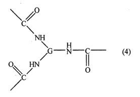
wherein G is a linear or branched  $C_3-C_{24}$  aliphatic trivalent radical, a  $C_5-C_{45}$  cycloaliphatic or aliphatic-cycloaliphatic trivalent radical, or a  $C_3-C_{24}$  aromatic or araliphatic trivalent radical;
