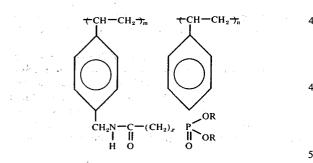
where R is an alkyl group having about 1–6 preferably about 2–4, carbon atoms and the copolymers contain about 0.1 to 10.0, preferably about 4.0 to 8.0 wt. pct. phosphorus. The phosphorus group is bonded to the phenyl group by an intervening methylene-amido alkyl group and said polystyrene copolymer is substantially non-crosslinked and has the properties of being flameresistant and char-forming when subjected to a flame.
