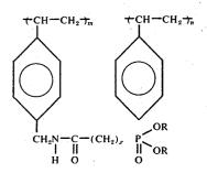
where R is an alkyl group having 1 to 6 carbon atoms, and the copolymer contains 0.1 to 10 wt. pct. phosphorus. The phosphorus group is bonded to the phenyl 60 group by an intervening alpha-amido methyl group and said polystyrene copolymer is substantially non-crosslinked.
