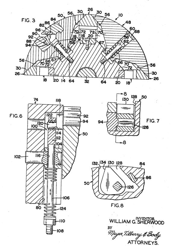
TENSION REEL GRIPPER MECHANISM
