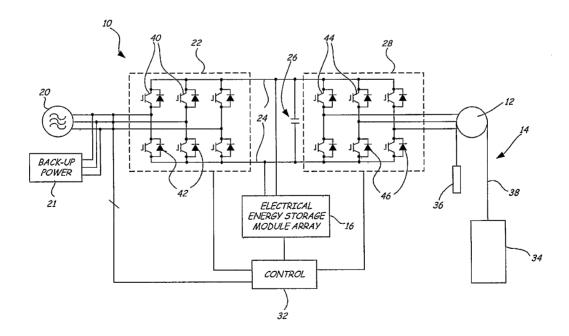
(57) Abstract: An elevator hoist motor (12) is driven by electrical energy storage (EES) modules (16) that are controlled such that at least one EES module drives the hoist motor (12) and at least one EES module charges. Subsequently, a controller (32) changes the at least one EES module that is driving the hoist motor (12) and the at least one EES module that is charging.
