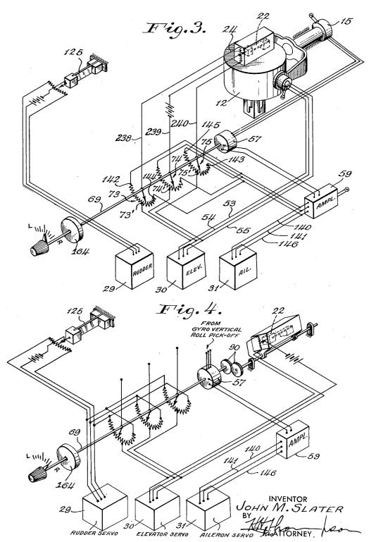
FLIGHT CONTROL APPARATUS FOR AIRCRAFT
