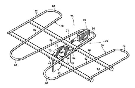
(57) **Abstract:** A magnetic centerguide (70) for a grid (40) structured for travel along a path of a conveyor (20). The grid defines a support surface that supports a pan (31-39). The guide comprises a magnet-carrying guide member (90) mounted on the grid.
