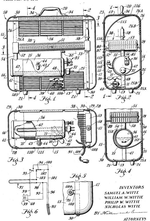
S. A. WITTE ET AL ELECTRICALLY HEATED FAN-RADIATOR APPARATUS
