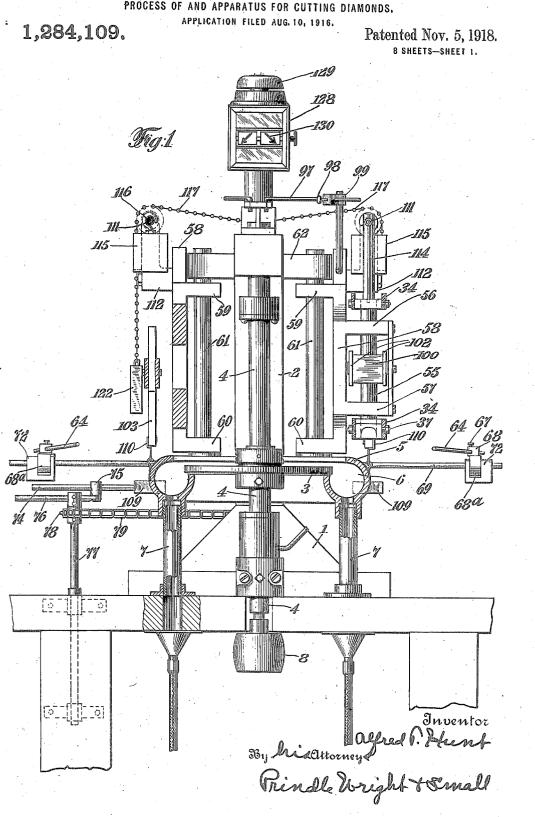
A. T. HUNT. PROCESS OF AND APPARATUS FOR CUTTING DIAMONDS.
