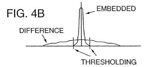
MEAN-REMOVED HISTOGRAMS OF FIRST DERIVATIVES (OR SCALER GRADIENTS IN THE CASE OF AN IMAGE)
