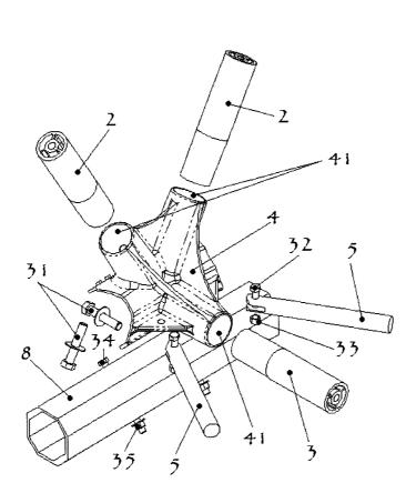
(57) Abstract: The present invention is directed toward a novel moment resisting connection system, for use, but not limited to, with a pony-truss bridge system. The connection system comprises multi-hollow sections that can be, but are not limited to, extruded aluminum and a joint or node connector that can be casted, milled, forged or made by any other means.
