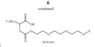
where R depicts C12–C13 alkyl groups. The reaction proceeds readily at ambient temperature and is exothermic. Use of the reaction product in preparing polyurethane foam provides for improved dimensional stability and cell opening.
