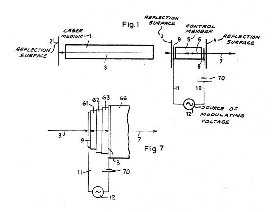
DEVICE FOR INTERNAL MODULATION OF LASER RADIATION
