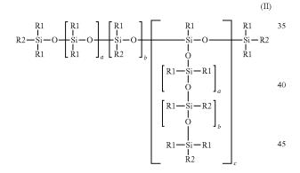
wherein: R1 is methyl; R2 is R1 or H, provided that at least three radicals R2 of the organopolysiloxane of formula (II) are hydrogen; a is 10-500; b is 1-50; c is 0-5; and the vinylsiloxane of formula (III) is:
