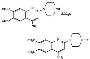
where Q is a facile leaving group, preferably Cl. The reaction is typically carried out by heating the reactants, preferably under reflux, in a suitable organic solvent, e.g. n-butanol, for up to about 24 hours, after which the product can be isolated conventionally.
