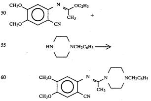
The crude product (26.9 g) from the previous Preparation, N-benzylpiperazine (21 g) and p-toluenesulphonic acid (100 mg) were stirred together at 150° for 2 hours under a slight pressure reduction. On cooling, the
