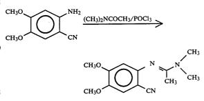
Phosphorous oxychloride (1.0 ml) was added to a stirred solution of dimethylacetamide (2.8 ml) in chloroform (10 ml) at room temperature. The mixture was so stirred for 5 minutes, 2-cyano-4,5-dimethoxyaniline (1.78 g) added and the reaction stirred under reflux for 4 hours. The mixture was cooled, poured onto ice and extracted with chloroform and the organic phase discarded. The aqueous layer was basified (solid NaOH)
