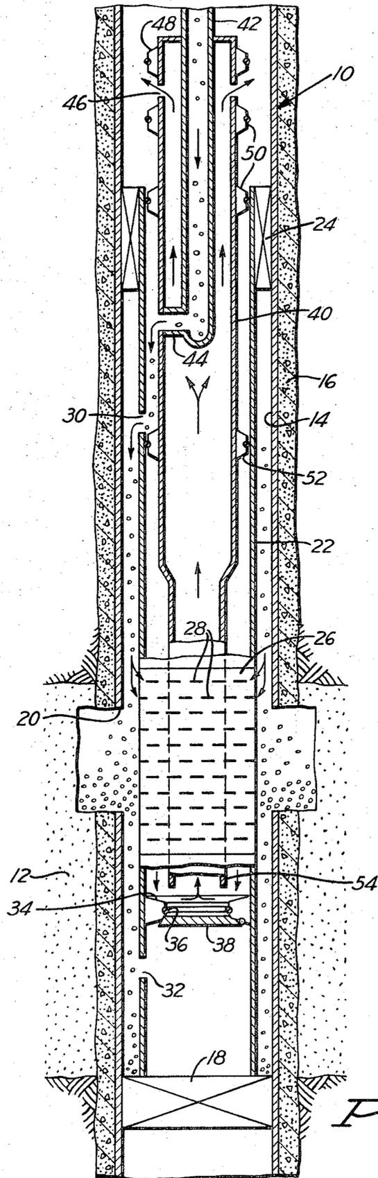
**GRAVEL PACKING METHOD AND APPARATUS**
