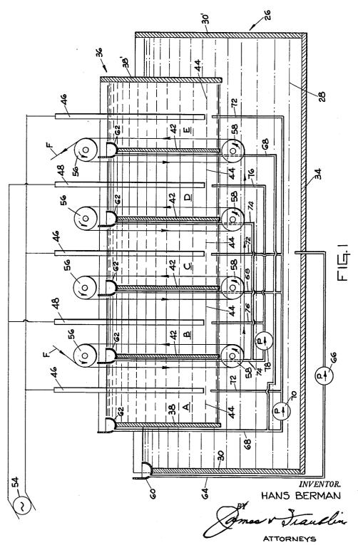
METHOD OF ANODIZING SLIDE FASTENERS
