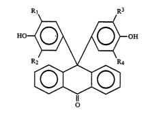
wherein  $R_1$ ,  $R_2$ ,  $R_3$  and  $R_4$  are independently hydrogen, lower alkyl of 1 to 4 carbon atoms or phenyl.
