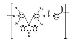
wherein  $R_1$ ,  $R_2$ ,  $R_3$  and  $R_4$  are independently hydrogen. lower alkyl of 1 to 4 carbon atoms or phenyl; n is the degree of polymerization; and wherein
