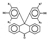
wherein R1, R2, R3 and R4 are independently hydrogen, lower alkyl of 1 to 4 carbon atoms or phenyl; or a polyarylate-forming derivative thereof; and a bisphenol compound selected from the group consisting of
