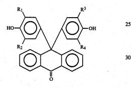
wherein R<sub>1</sub>, R<sub>2</sub>, R<sub>3</sub> R<sub>4</sub> are independently hydrogen, lower alkyl of 1 to 4 carbon atoms or phenyl; or a polyarylate-forming derivative thereof; and a bisphenol compound selected from the group consisting of
