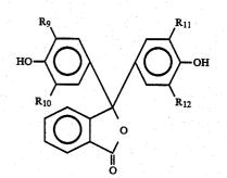
wherein  $R_9$ ,  $R_{10}$ ,  $R_{11}$  and  $R_{12}$  are independently hydrogen, lower alkyl or 1 to 4 carbon atoms or phenyl; and
