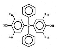
wherein R13, R14, R15 and R16 are independently hydrogen, lower alkyl of 1 to 4 carbon atoms or phenyl; and wherein the molar ratio of 5-keto-bis(hydroxyphenyl-50 )anthracene to bisphenol is from 20:1 to 1:20; and
