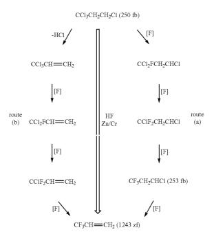
**[0057]** Alternatively, 250fb may be dehydrochlorinated to produce 3,3,3-trichloropropene, followed by step-wise fluorination to produce 1243zf. This is illustrated above as route (b).
