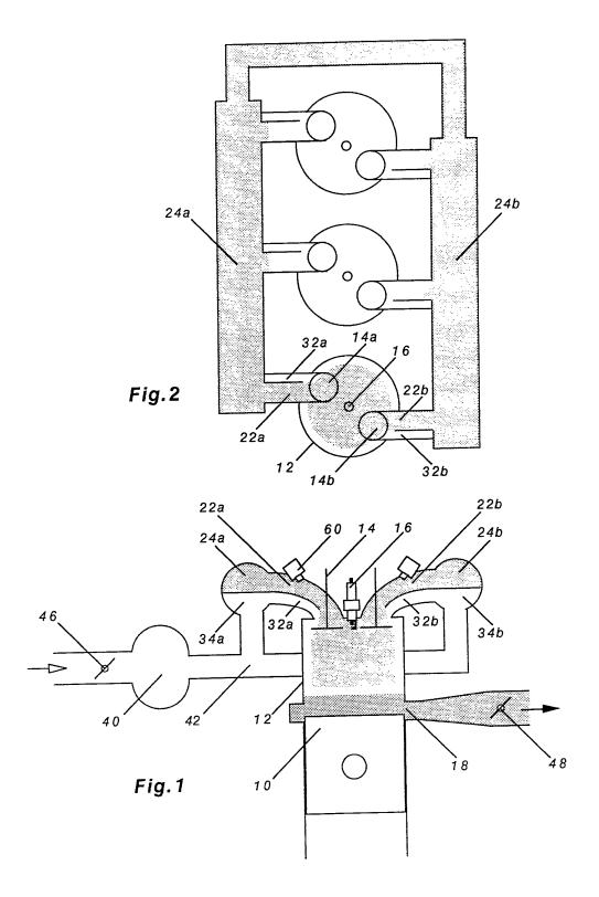
Intake Manifold System for a Two Stroke Engine
