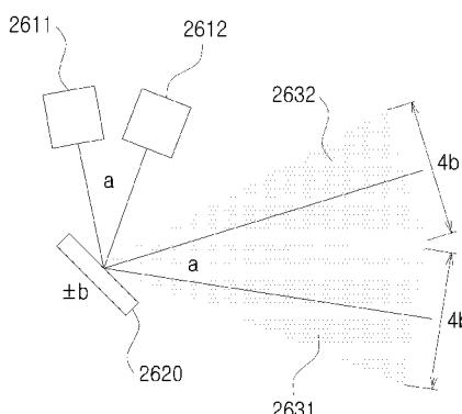
(57) Abstract: The present invention relates a lidar device that measures distance using a laser, the lidar device comprising: a first laser output unit for outputting a first laser; a second laser output unit for outputting a second laser; a scanning for forming a first viewing angle using the first laser and forming a second viewing angle using the second laser; and a detector for measuring the distance to an object using the first and second lasers.
