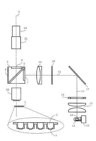
(57) Abstract: An epifluorescent imaging system is arranged to have an imaging axis (4) along which, in use, light travels between an optical element (5) comprising a dichroic mirror (6) and a sample position of a sample to be analysed. The imaging system comprises an illumination system, comprising a fitting (12) for a metal halide lamp (13). The epifluorescent imaging system comprises a metal halide lamp comprising a gas discharge tube (14), fitted in the fitting (12).
