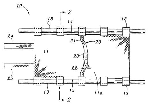
(57) Abstract: Transitional support (10) for physically challenged persons. The support (10) has a flexible inelastic base sheet (11) with flexible inelastic loops (12), (13) at parallel edges (14), (15) to accommodate removable rigid poles (18), (19). Pull straps (24), (25) on the sheet (11) may be included to pull a person along the floor. To provide for a sitting support, a back sheet (40) can be provided to join with the folded base sheet as a back restraint.
