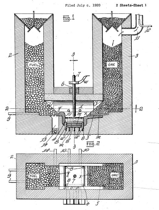
PROCESS OF ELECTRIC SMELTING AND FURNACE FOR SAME
