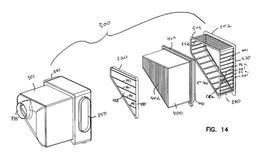
(57) Abstract: A media pack for including in a filter cartridge of an air filter arrangement, is provided. The media is a non-rectangular perimeter configuration, an example shown being trapezoidal. Filter cartridges including such media packs, air cleaner assemblies and equipment systems are described. Also methods of use assembly are described.
