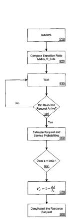
(57) Abstract: A method of controlling a resource management system by modeling the resource management system with a Markov process. The transition probabilities used in the Markov model are determined by making empirical measurement of the distribution of the actual system and using actual statistic to estimate the transition probabilities. The transition probabilities are constantly modified based upon a feedback control measurement system per Fig 9.
