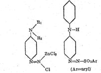
In the alternative, the diazo compounds may be of the passive type which are light-sensitive but which are activated only in acidic medium for reaction with a coupler to form an azo dyestuff. These include diazo compounds of the type described in the copending application Ser. No. 316,948 such as the metallic salts of the acid isomeric forms of the diazo compounds, including the isodiazotates or nitrosoamines or the diazo amino or diazo imino compounds represented by the formula
