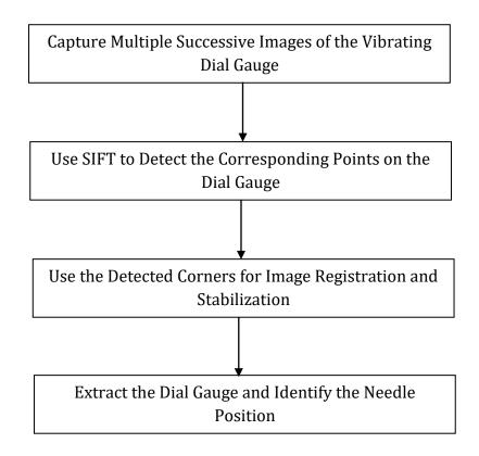
Figure - 4: Flow chart to obtain the gauge reading even when it is Vibrating
