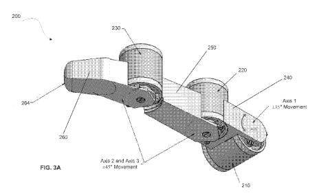
(57) Abstract: A robotic finger, comprising: a first axis of movement comprising a moving magnet; a second axis of movement comprising a moving coil, wherein the second axis is generally orthogonal to the first axis; and a third axis of movement comprising a moving magnet, wherein the third axis of movement is generally oriented in the same direction as the first axis of movement.
