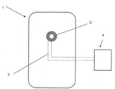
(57) Abstract: A trim component comprising a decorative layer and an electrical circuit path positioned on the B (i.e., back or hidden) surface of the decorative layer, the electrical circuit path comprising conductive ink/paint in a geometric configuration suitable for transmitting wireless power. The trim component can further comprise a protective layer positioned such that the electrical circuit path is at least partially enclosed between the decorative layer and the protective layer.
