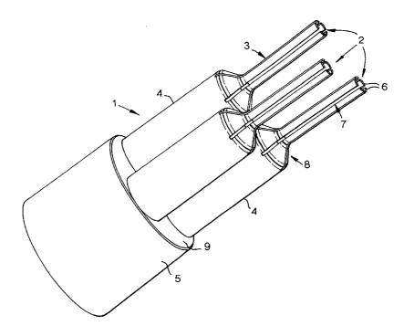
(57) Abstract: A device (1) for applying radially expandable and recoverable sleeves (12) on elongate articles (11), such as cables, is arranged for expanding the sleeves (12) upon insertion of the elongate articles (11) into the device (1). The device (1) comprises two or more expandable substantially tubular sections (2) allowing two or more sleeves (12) to be expanded simultaneously.
