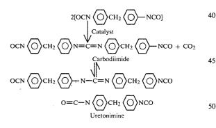
Examples of commercial materials of this type are Upjohn's ISONATE (R)125M (pure MDI) and ISONA-TE (R)143L ("liquid" MDI). Preferably the amount of 55 isocyanates used is the stoichiometric amount based on all the ingredients in the formulation or greater than the stoichiometric amount.
