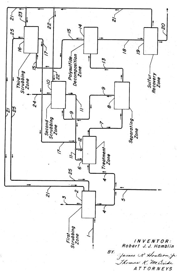
July 20, 1971 REMOVAL AND RECOVERY OF SULFUR FROM A GAS STREAM CONTAINING H<sub>2</sub>S Filed Feb. 26, 1969
