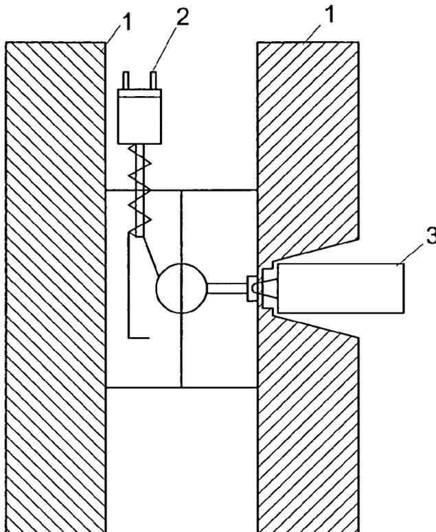
(57) Abstract: Apparatus for carrying out multicomponent injection-moulding processes, in particular two-component injection-moulding processes, characterized in that one or more further plastifying unit(s) has/have been integrated in the mould.
