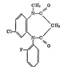
was prepared from 5-(2'-fluoro-phenyl)-7-chloro-1H,1,5-15 benzodiazepin-2,4-(3H,5H)-dione and methyl iodide.
