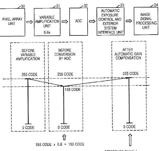
153 CODE x REFERENCE GAIN(IX) = 255 CODE AMPLIFICATION UNIT(0.6x)
