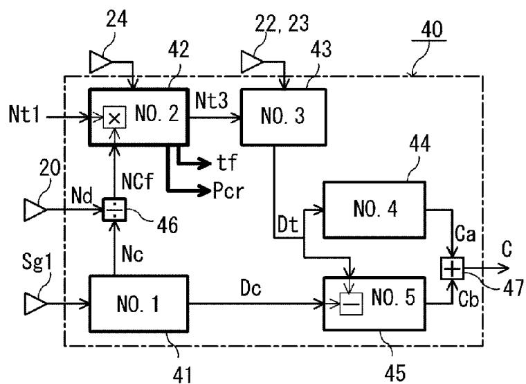
(57) Abstract: A control device 30 is configured in such a way that if the operating state of an engine 10 is a state of acceleration, while under EGR control for suppressing the generation of smoke, a fuel injection timing  $t_f$  for injection of fuel into a cylinder is delayed, and/or a fuel injection pressure  $P_{cr}$  is reduced, without increasing a NO<sub>x</sub> concentration target value  $N_{t1}$  set on the basis of the operating state of the engine 10.
