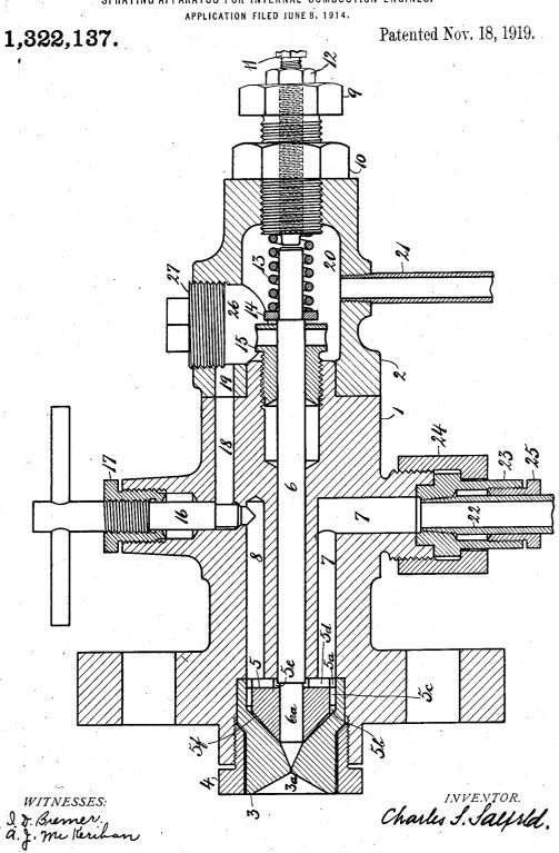
C. S. SALFELD. SPRAYING APPARATUS FOR INTERNAL COMBUSTION ENGINES.
