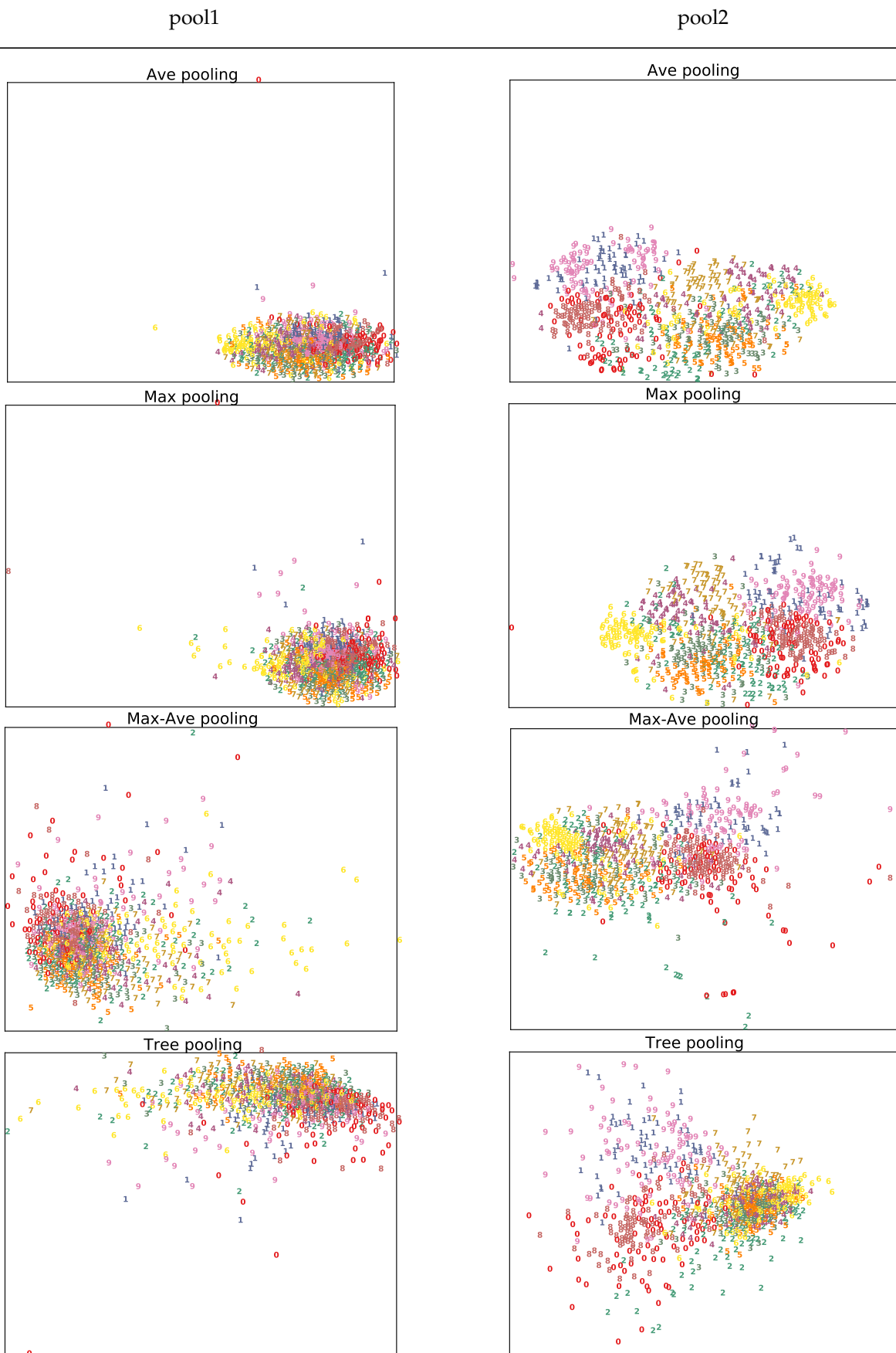
Fig. 6: t-SNE embeddings of the output responses from different pooling operations on the CIFAR10 test set (with classes indicated). From top to bottom: average, max, gated max-avg, and (2 level) tree pooling. The first and the second columns show the first and the second pooling layers, respectively. Best viewed in color.
