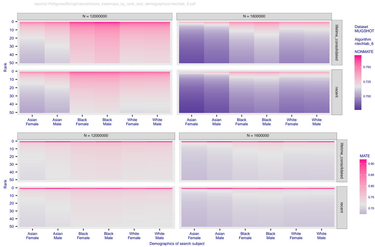
Figure 26: For searches of Asian, black, white men and women’s faces into mixed galleries of mugshot photos the heatmaps show median similarity scores for candidates placed at rank 1 to 50. The upper four panels are produced in nonmated searches; the lower four from mated searches. The left-side panels are produced from searches into galleries with 12 000 000 people enrolled. The right-side uses galleries with N = 1 600 000 enrolled. The “lifetime consolidated” and “recent” labels refer to inclusion of multiple images per person, or just one - see [17]. Contrast the behavior here with that in Figure 27 and the corresponding figures for developers Aware, Idemia, NEC, Tevian, and Toshiba that are included in Annex 17 .
